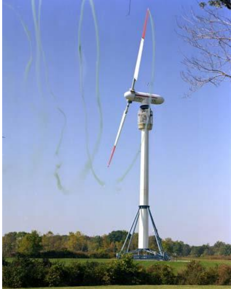
Figure 1. Smoke experiment by NASA on an experimental wind turbine
