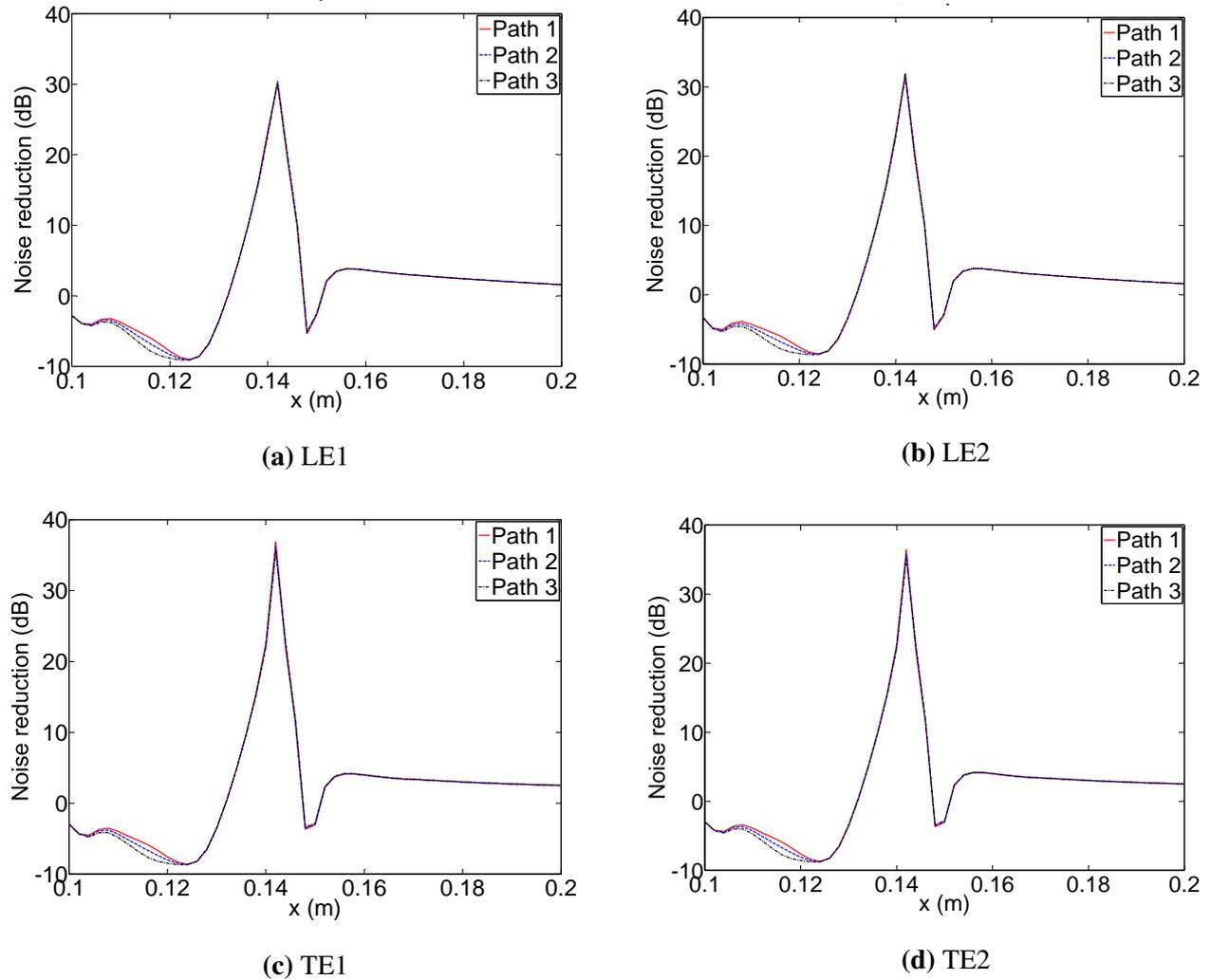
Figure 3 – Noise reduction using serrated trailing edge as a function of quadrupole location along the x-direction for three different paths at 500 Hz
