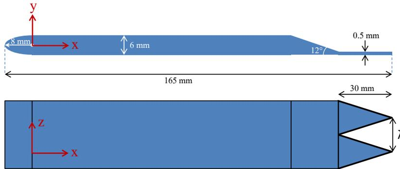
Figure 1 – Dimensions of the flat plate with serrated trailing edge
