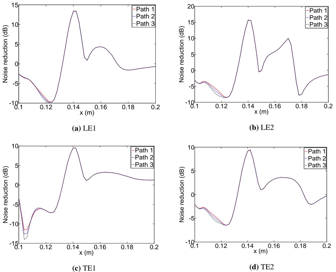
Figure 4 – Noise reduction using serrated trailing edge as a function of quadrupole location along the  $x$ -direction for three different paths at 2000 Hz
