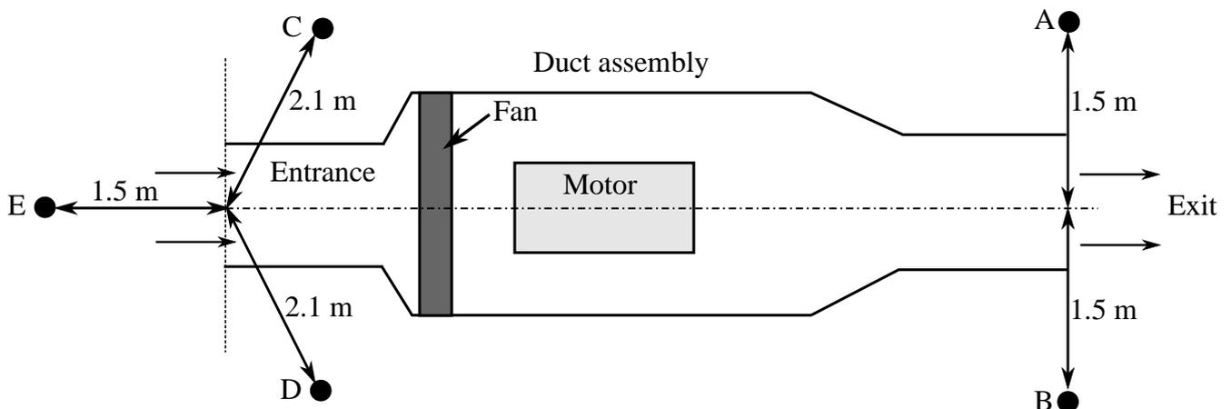
(b) Schematic diagram showing microphone positions
