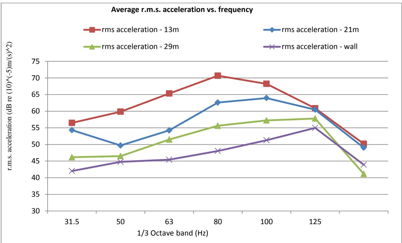
Figure 7. Average r.m.s. acceleration vs 1/3 octave band
