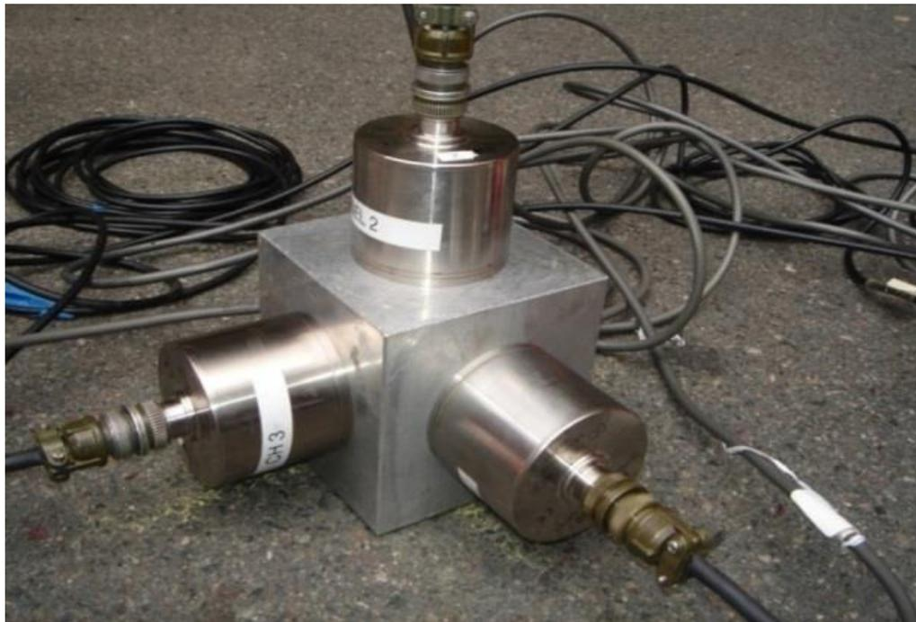
Figure1. Tri-axial accelerometer setup [2]
