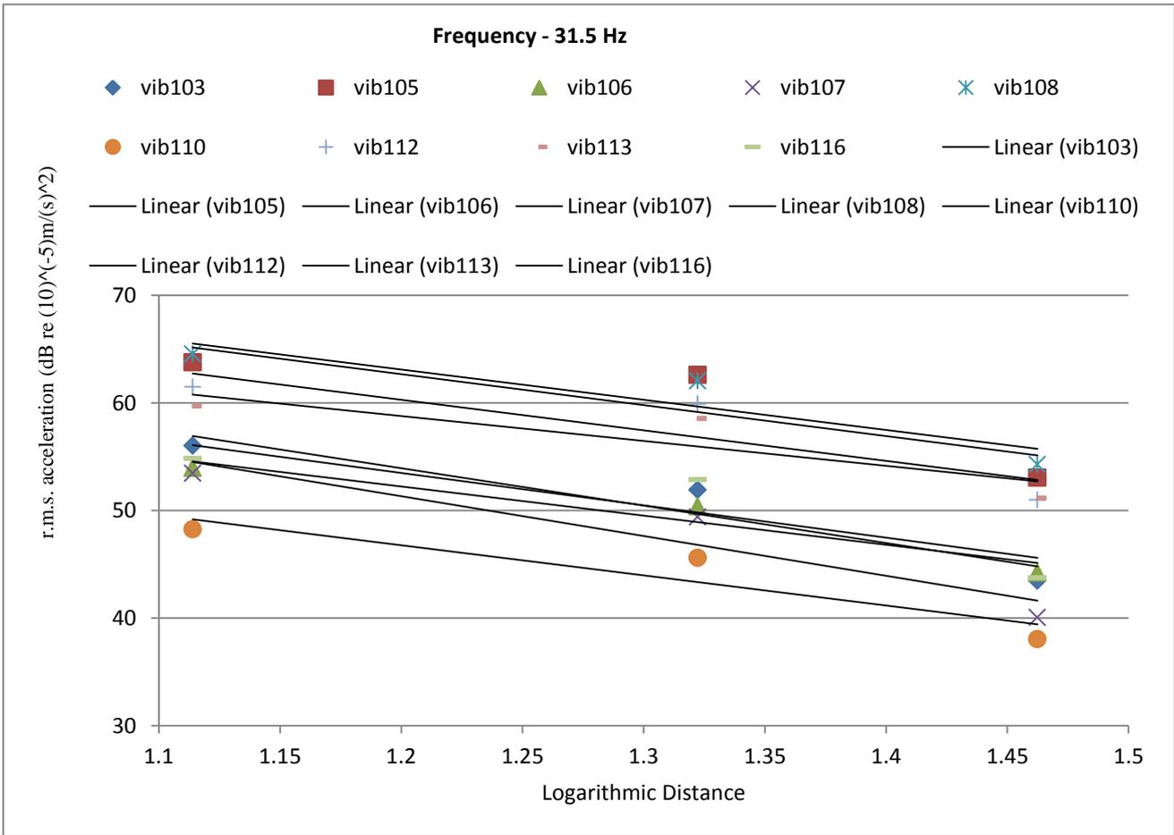
Figure 8. Average r.m.s. acceleration vs logarithmic distance (31.5Hz)
