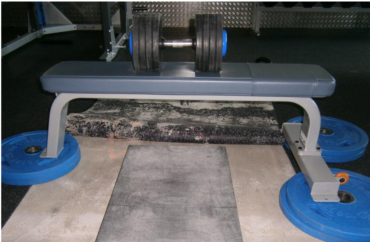
Figure 4. Test setup showing the 42.5kg dumbbell and 420mm high weights bench
