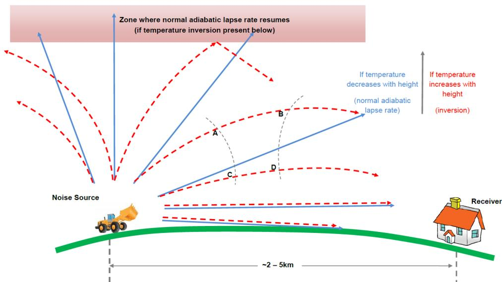
Figure 2. Influence of temperature inversions on propagation of noise
