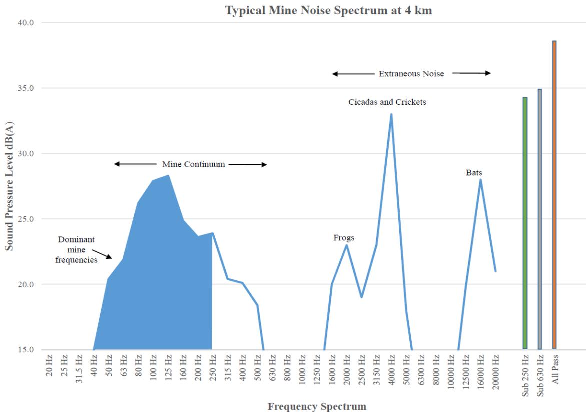
Figure 4. A typical spectral signature of a large open cut mine at around 4km.
