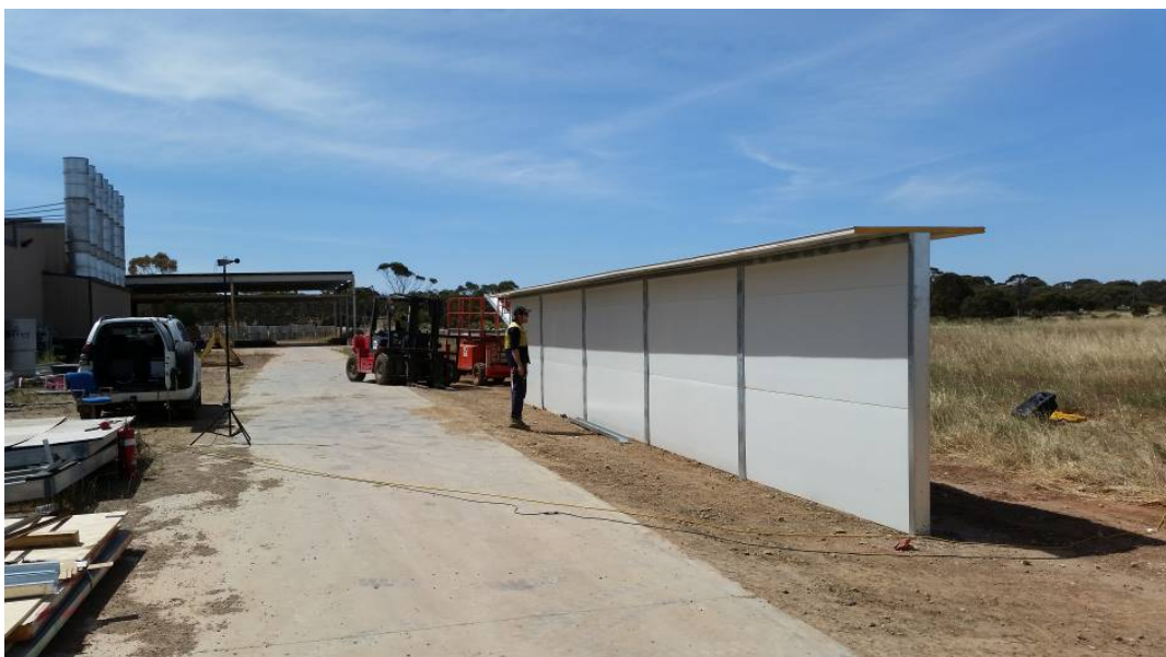
Figure 4. 2.4 m high 600 mm wide T-profile barrier installed at test site with microphone at 2.5 m high above ground and loudspeaker on opposite side of barrier.
