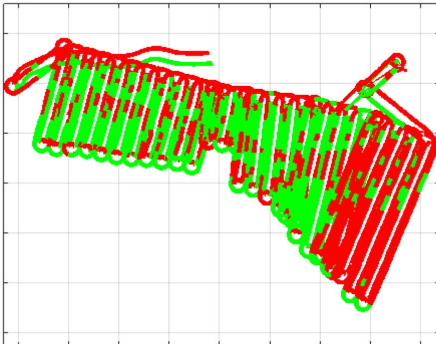
Figure 6. Classification of seabed as even textured or as rough (including artefacts). Red areas have more than 3% rough pixels, green areas have less than 3%. Red images at the ends of north-south sections correspond to image distortions caused by turns. In the west the quasi-zonal band along the centre of the surveyed area is caused by image distortions from terrain following height adjustments over a steep slope. The red eastern area corresponds to dark imagery with little information.
