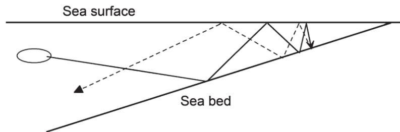
Figure 4. Schematic of sonar termination. An acoustic signal directed into a wedge may experience many seabed and sea surface reflections, becoming greatly attenuated and distorted before, and if, it returns to the transmitter.
