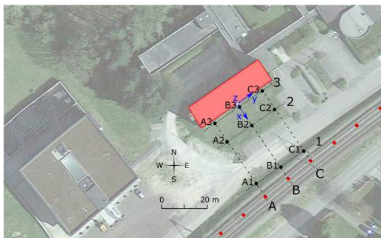
Figure 2: Free field measurement locations (black dots). The measurement lines A, B, and C correspond to y = -12 m, y = 0 m and y = 12 m, respectively. The measurement lines 1, 2, and 3 correspond to x = 32 m, x = 12 m, and x = 1 m, respectively. Eight of the seventeen hammer impact locations are also shown (red dots).
