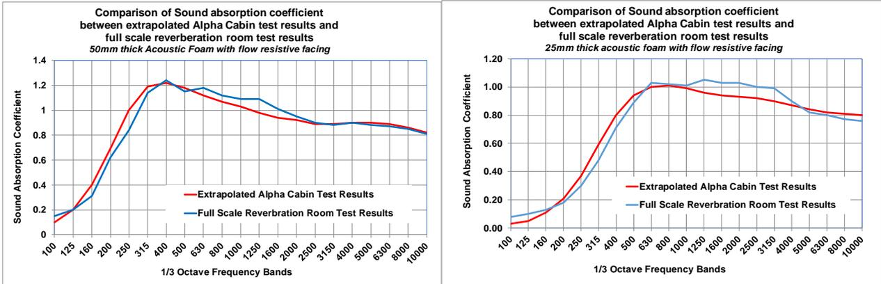
Figure 5: Comparing full scale test results with computed data based on Alpha Cabin measurements
