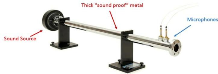
Figure 2. An example of Impedance tubes
