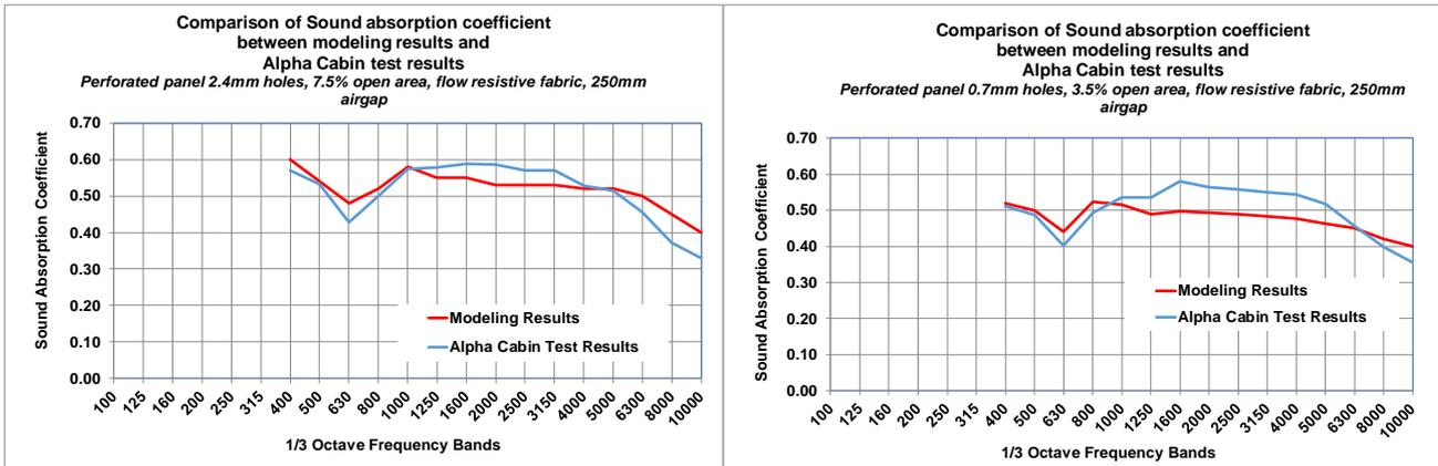
Figure 8: Modelling perforated panels with flow resistive facing based on test results obtained from the Alpha Cabin
