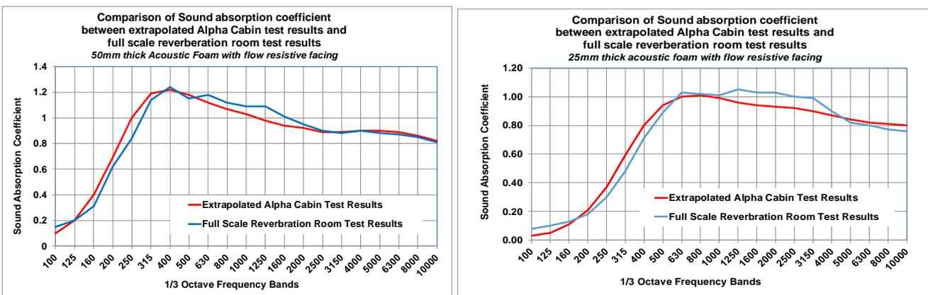
Figure 7: Comparing full scale test results with computed data based on Alpha Cabin measurements
