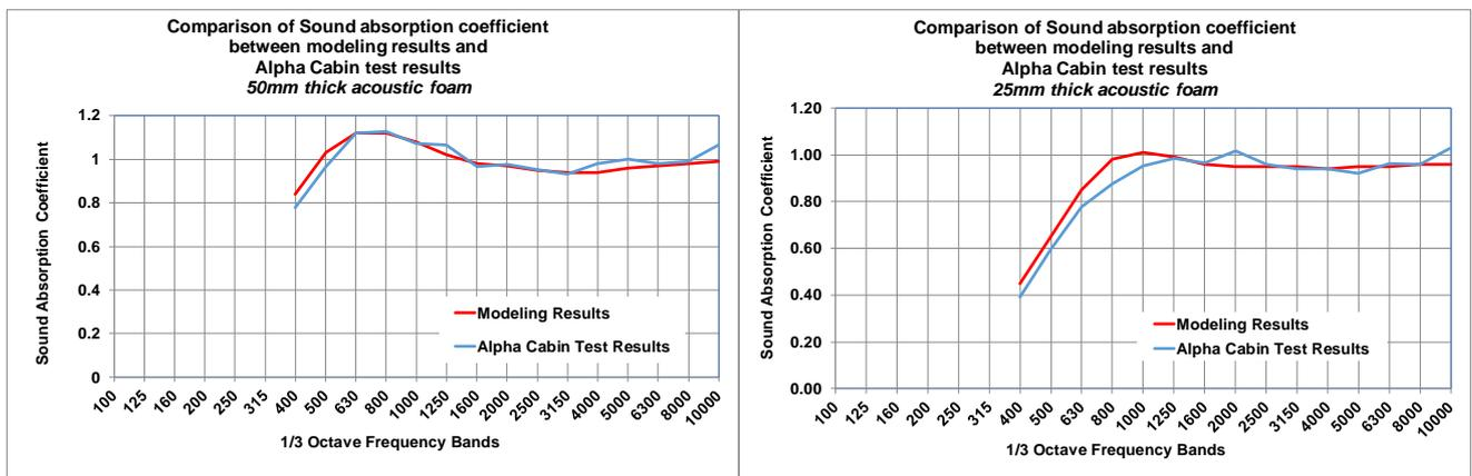
Figure 4: Modelling plain acoustic foam based on test results obtained from the Alpha Cabin
