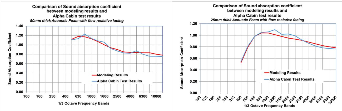
Figure 6: Modelling acoustic foam with flow resistive facing based on test results obtained from the Alpha Cabin
