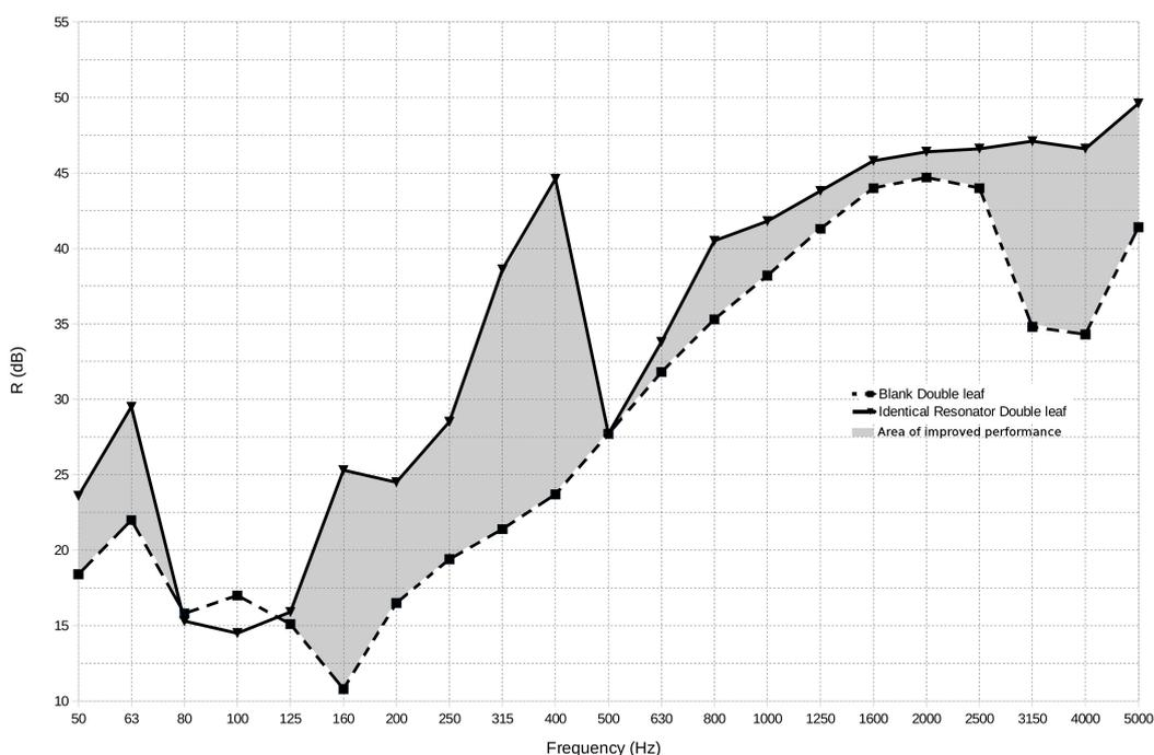
Figure 7: This figure shows the diffuse field results of the SRLRS without absorption material
