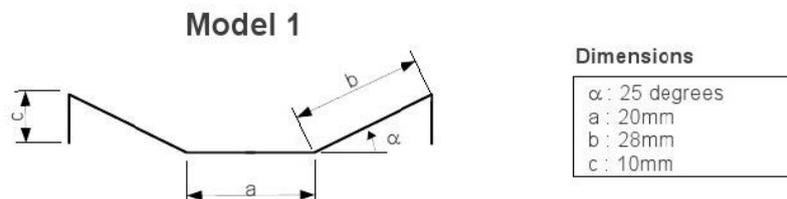
Figure 5: This figure shows the dimensions of the diffuse field resonator
