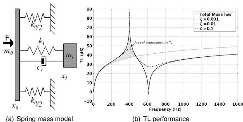
Figure 1: Spring-mass model and an example of a TL vs Frequency performance plot for a single layer LRS
