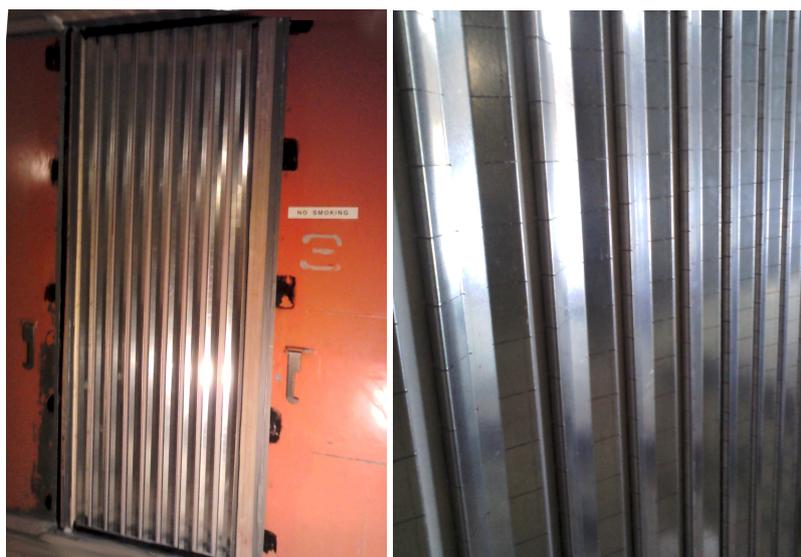
(a) One side of full scale wall (b) Resonators on metamaterial wall
