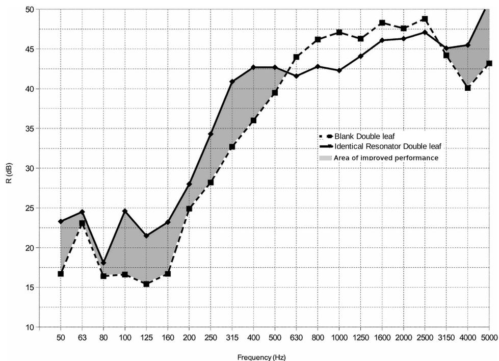
Figure 10: The diffuse field results of the MAMCLRS with absorption material in the cavity
