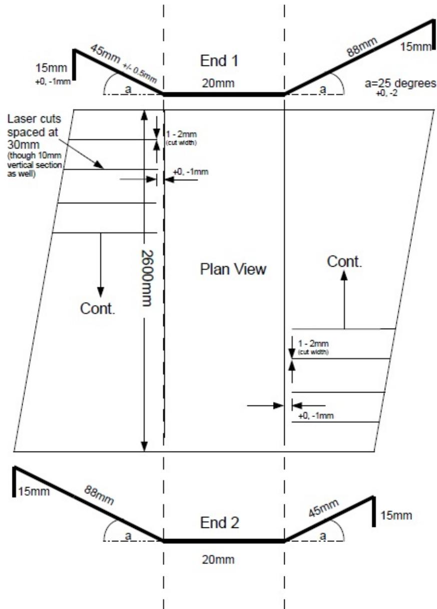
Figure 8: The dimensions of the diffuse field resonator
