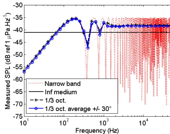
Figure 3: Received level (dB) from a source 4 m below the surface observed at a range of 100 m and a slant angle of  $30^\circ$ .
