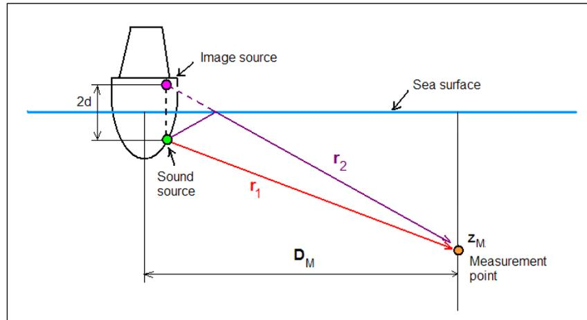
Figure 1: The Lloyd's mirror effect in relation with ship radiated noise.
