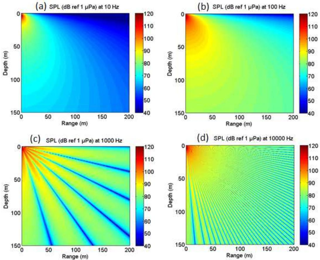
Figure 2: Map of SPL from a point source below sea surface acting as a perfectly reflecting mirror for different frequencies and  $d = 4$  m : (a) 10 Hz, (b) 100 Hz, (c) 1000 Hz and (d) 10000 Hz.
