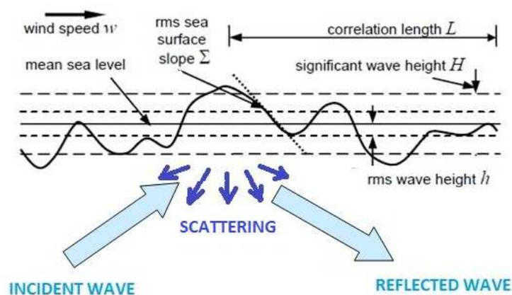
Figure 5: Reflection and scattering of underwater acoustic waves on a rough sea surface.
