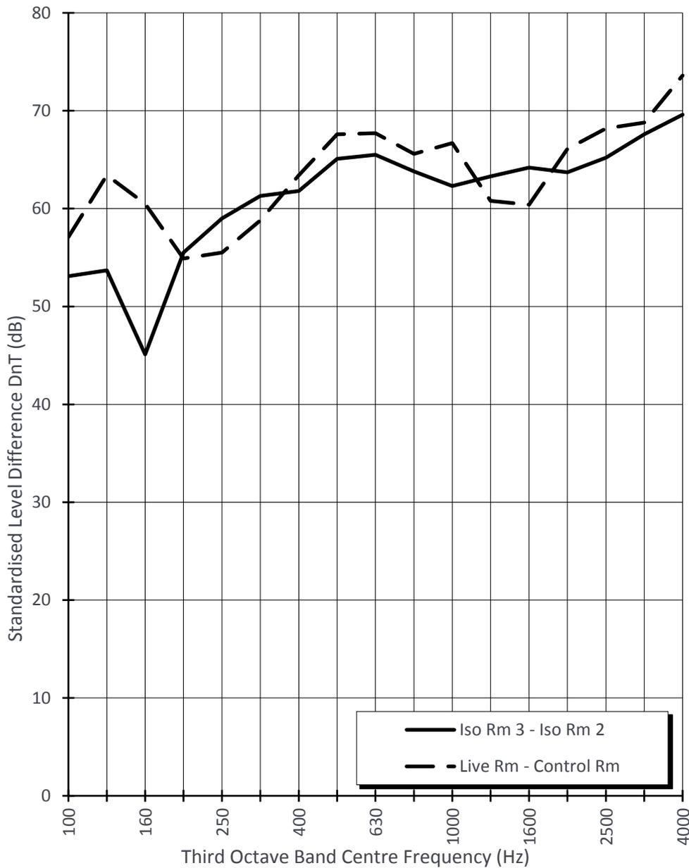
Figure 5: Transmission Loss tested on completion
