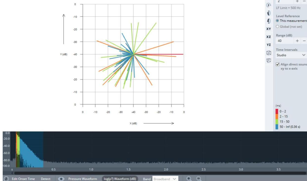
Figure 4: IRIS 3D impulse response (XY plane) in Control Room 1 from RHS monitor location
