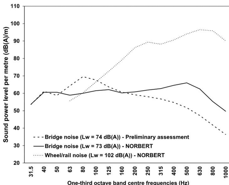
Figure 3: Predicted noise spectra based on preliminary and NORBERT assessments
