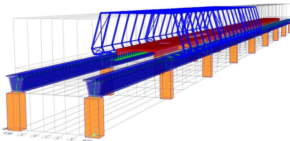
Figure 4: FE model of the elevated station platform used in the case study
