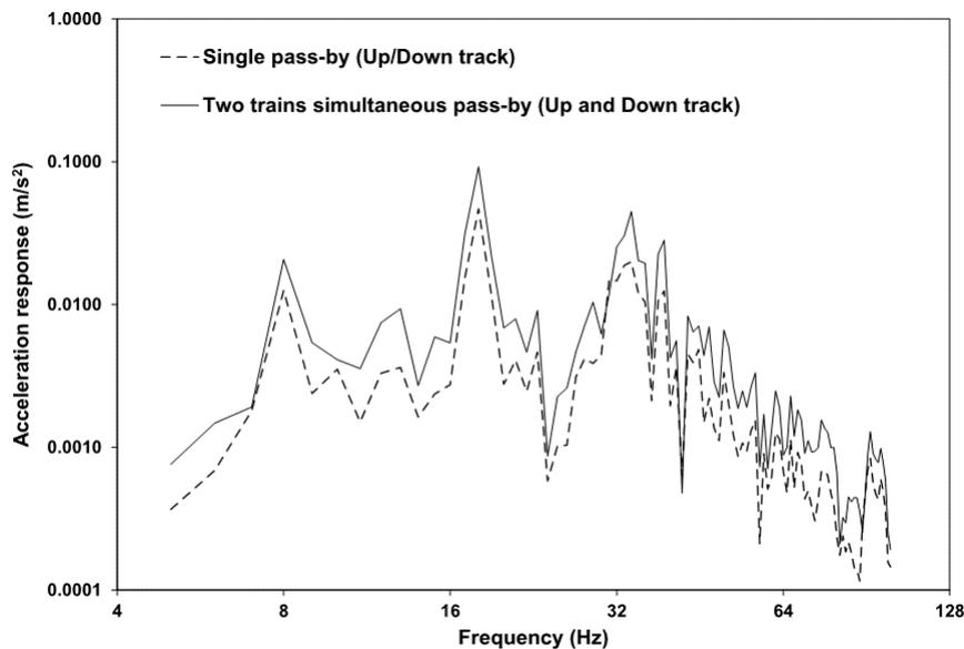
Figure 5: Acceleration response prediction on elevated station platforms (on worst-affected node)
