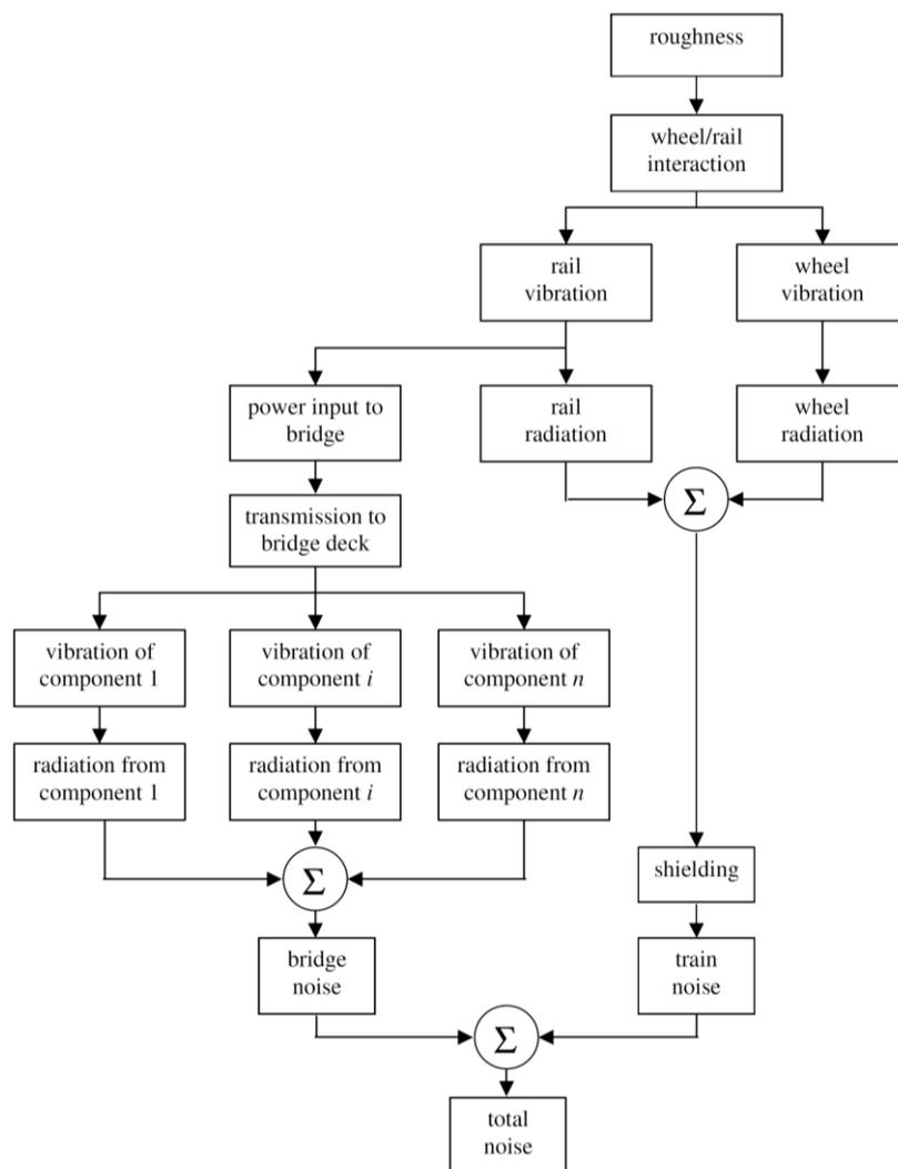
Figure 1: Flowchart explaining the elements considered in NORBERT modelling
