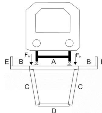
Figure 2: Schematic of the box girder cross-section
