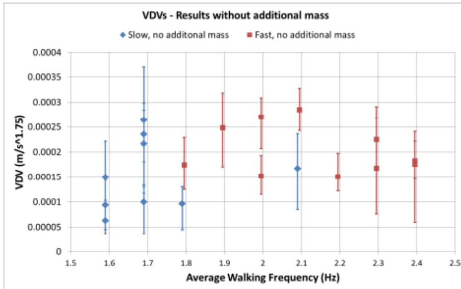
Figure 2: VDV Results versus Stepping Frequency (no additional mass).
