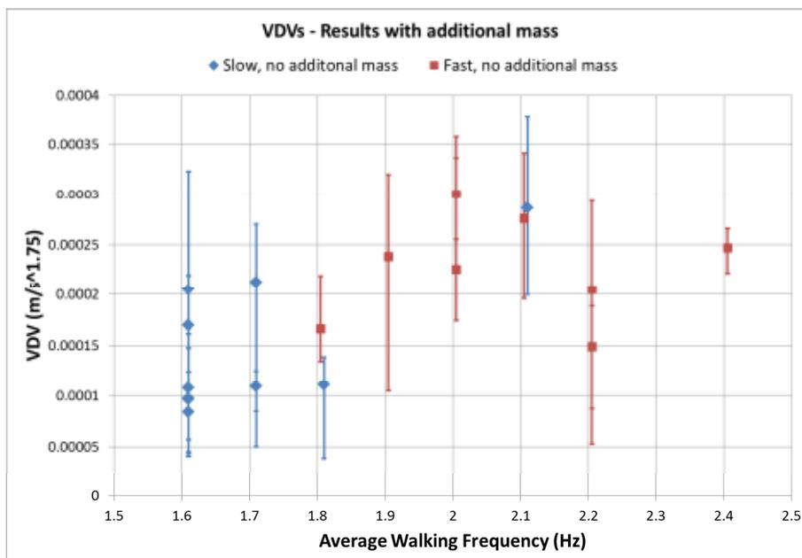
Figure 3: VDV Results versus Stepping Frequency (with additional mass).
