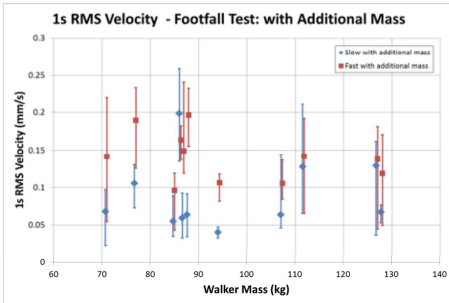
Figure 11: 1s RMS Velocity Results – with Additional Mass
