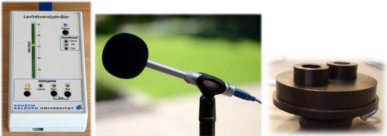
Figure 3: Left: The low-frequency measurement device with a simple user interface (in Danish).
