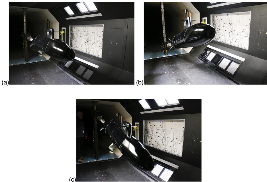
Figure 1: Photographs of the model and the 64 microphone array in the wind-tunnel with a zero (a), positive (b) and negative (c) pitch angle.
