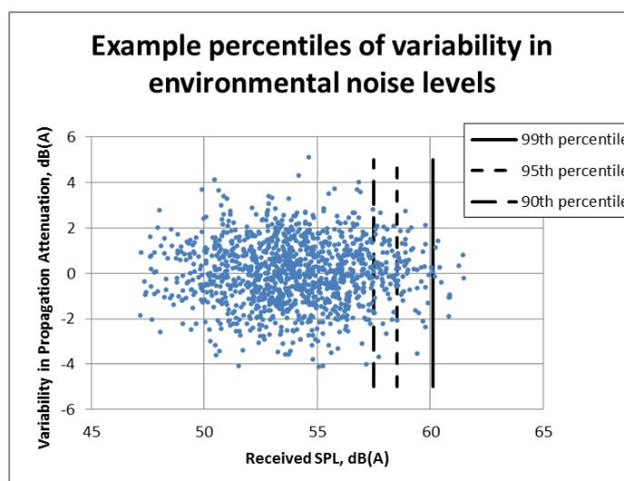
Figure 8: Example percentiles of received noise level samples
