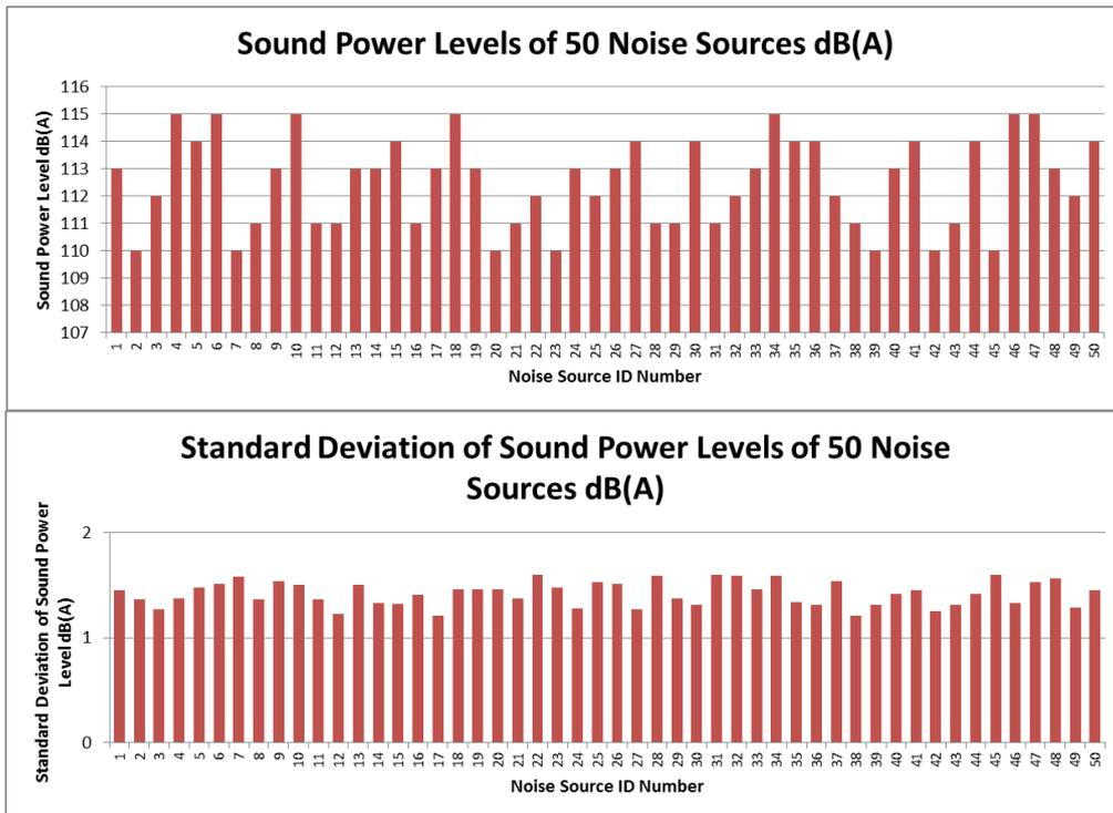
Figure 9: Example sound power levels and standard deviations of 50 noise sources
