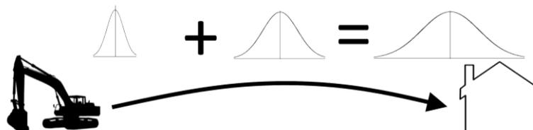
Figure 3: Received SPL variability due to the combination of source emission variability and propagation variability
