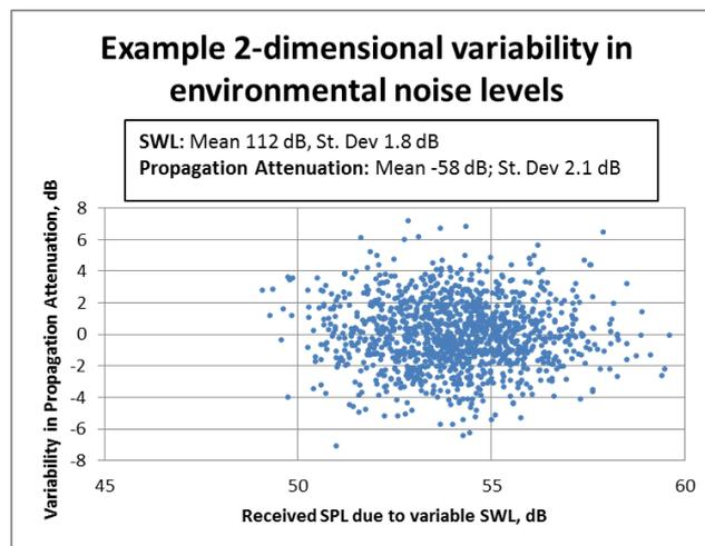
Figure 6: Scatter plot of example variability in noise received due to variable noise source noise emissions and variable propagation attenuation
