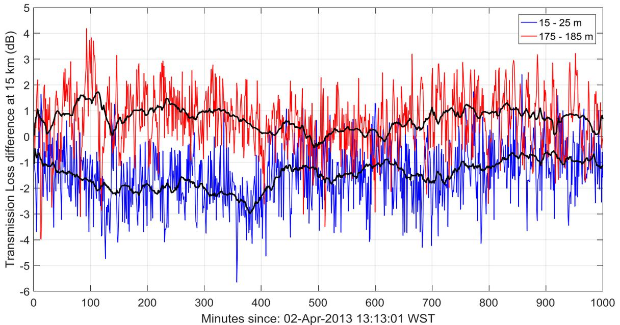
Figure 5: The difference in the modelled transmission loss obtained using the range dependent SVP minus the results obtained using range independent modelling based on the SVP at the source at each time. The black lines are 50 minute median filter versions.
