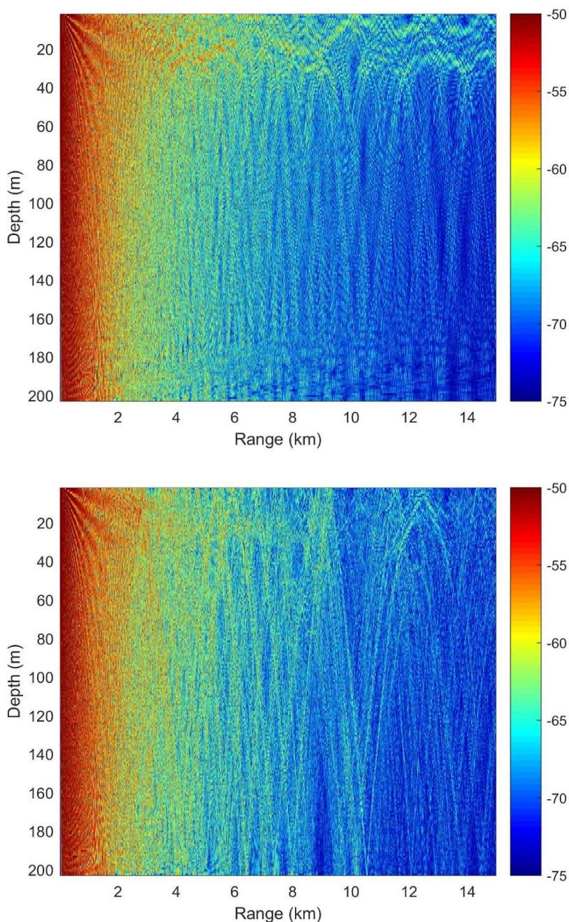
Figure 6: Transmission loss as a function of depth and range using range independent SVP (top), and range dependent SVP (bottom) at 7 pm on 2<sup>nd</sup> Apr-2013 (WST).
