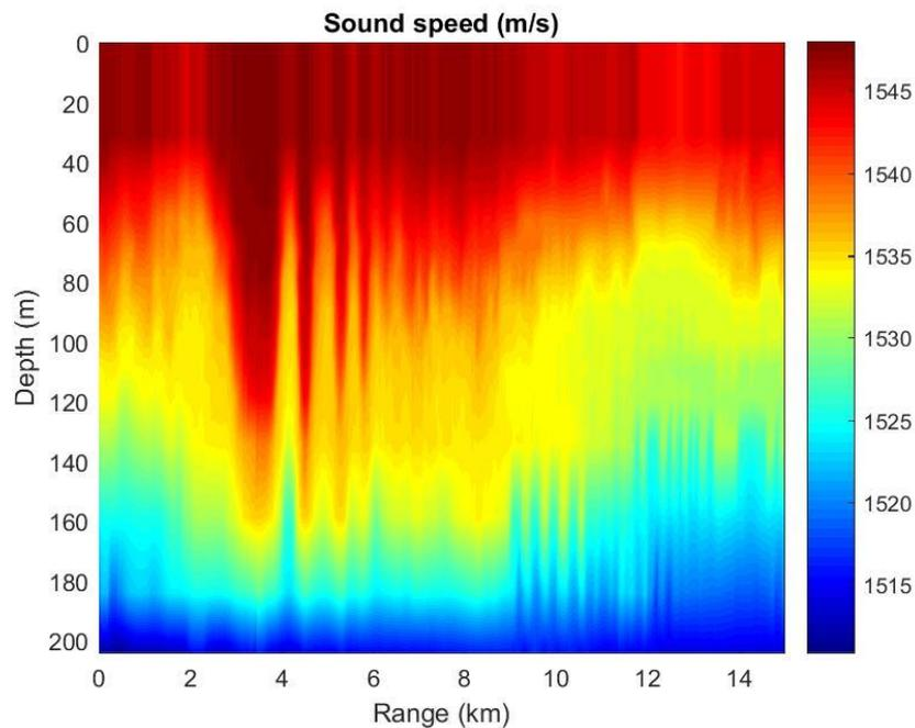
Figure 7: Sound velocity profiles (m/s) used in modelling Figure 6. Range independent (top) and range dependent (bottom).
