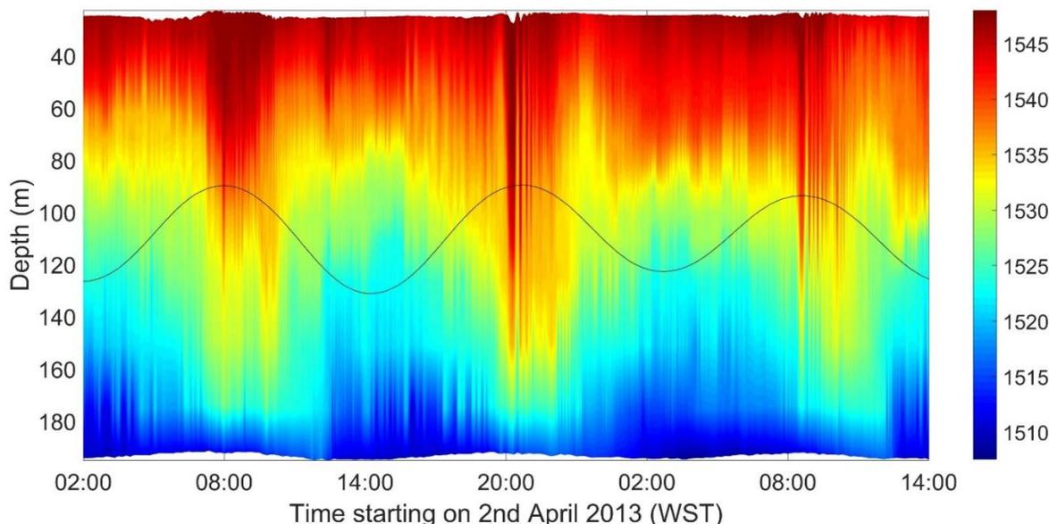
Figure 2: Sound velocity profiles (colour plot) and relative predicted tide (black line) between 2<sup>nd</sup> and 3<sup>rd</sup> April 2013 calculated from the CTD data collected on the 200 m IMOS mooring off the Kimberley coast, Western Australia.
