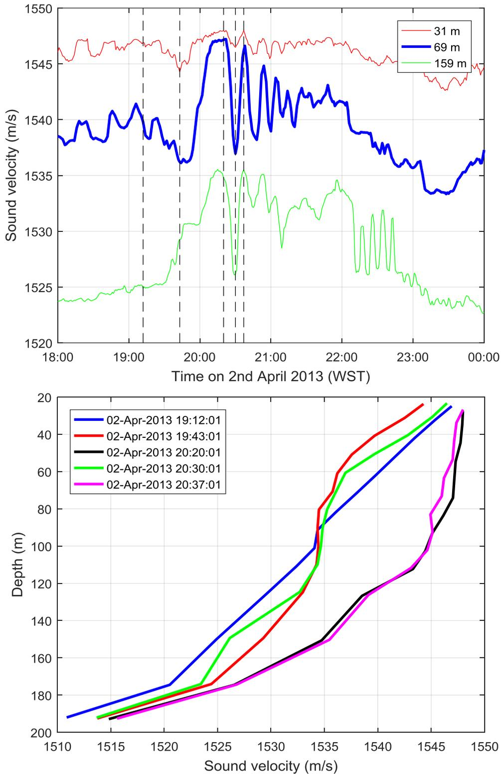
Figure 3: Sound velocity vs time at selected depths (top), with vertical black dashed lines showing the times of SVP profiles (bottom), during 2<sup>nd</sup> April 2013. Data is from the 200 m mooring.
