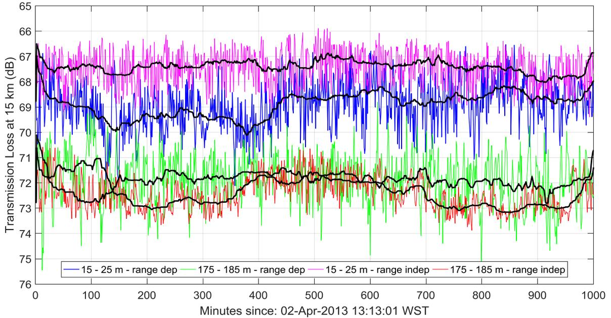
Figure 4: Modelled transmission loss at a range of 15 km as a function of time for receivers near the sea surface and the seafloor. The blue and green curves shows the results obtained using the appropriate range dependent SVP at each time, whereas the magenta and red curves show the results obtained using range independent modelling based on the SVP at the source at each time. The black lines are 50 minute median filter versions.
