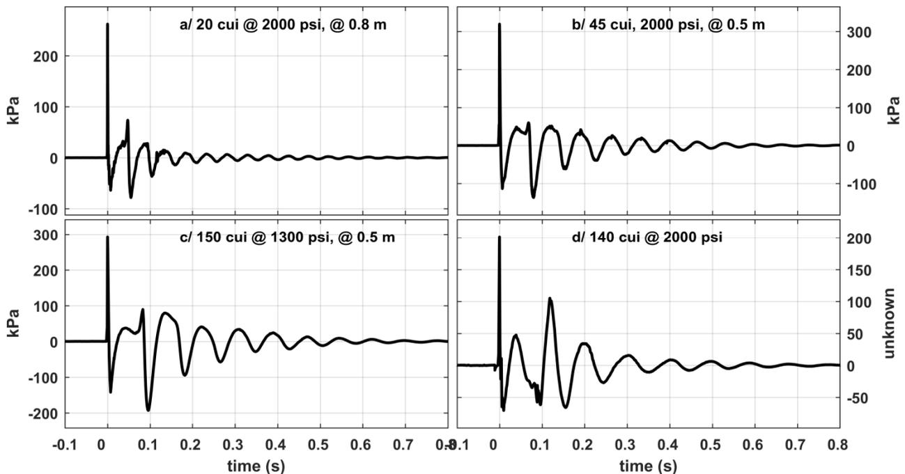
Figure 1: Images of single air gun waveforms (a/ to c/) and a gun cluster (d/, a 20 and 3 x 40 cui guns arranged in a 1.3 x 1.11 m rectangle, with the hydrophone located at the forward end with a 20 and 40 cui inch gun adjacent and recorded with an uncalibrated hydrophone). All sources were at 5-6 m depth.
