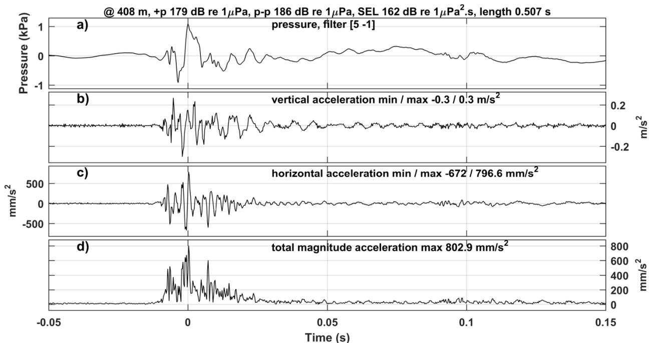
Figure 2: A single seismic signal as recorded at 408 m from a 150 cui air gun in 10 m water depth over a sandy seabed, showing: a) the pressure waveform at the seabed; b) the vertical ground acceleration; c) the horizontal ground acceleration; and d) the magnitude of the total ground acceleration.
