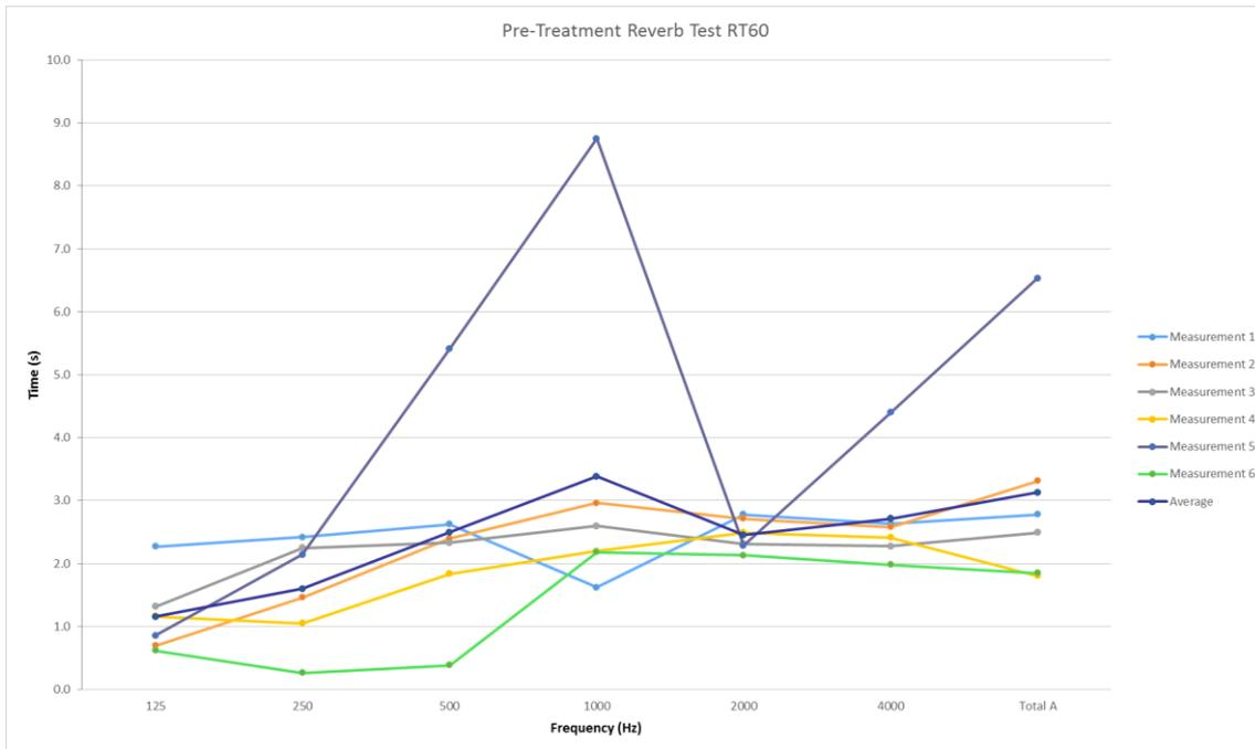
The graph above shows the results of the measured RT60 data in seconds. The overall average was calculated to be 3.1 seconds. Measured reverberation time at location “Measurement 5” shows a large decay time of 8.7 seconds at the 1kHz and 5.5seconds at the 500Hz Octave bands. This was due to the glass windows, doors and water being the reflective surfaces.
