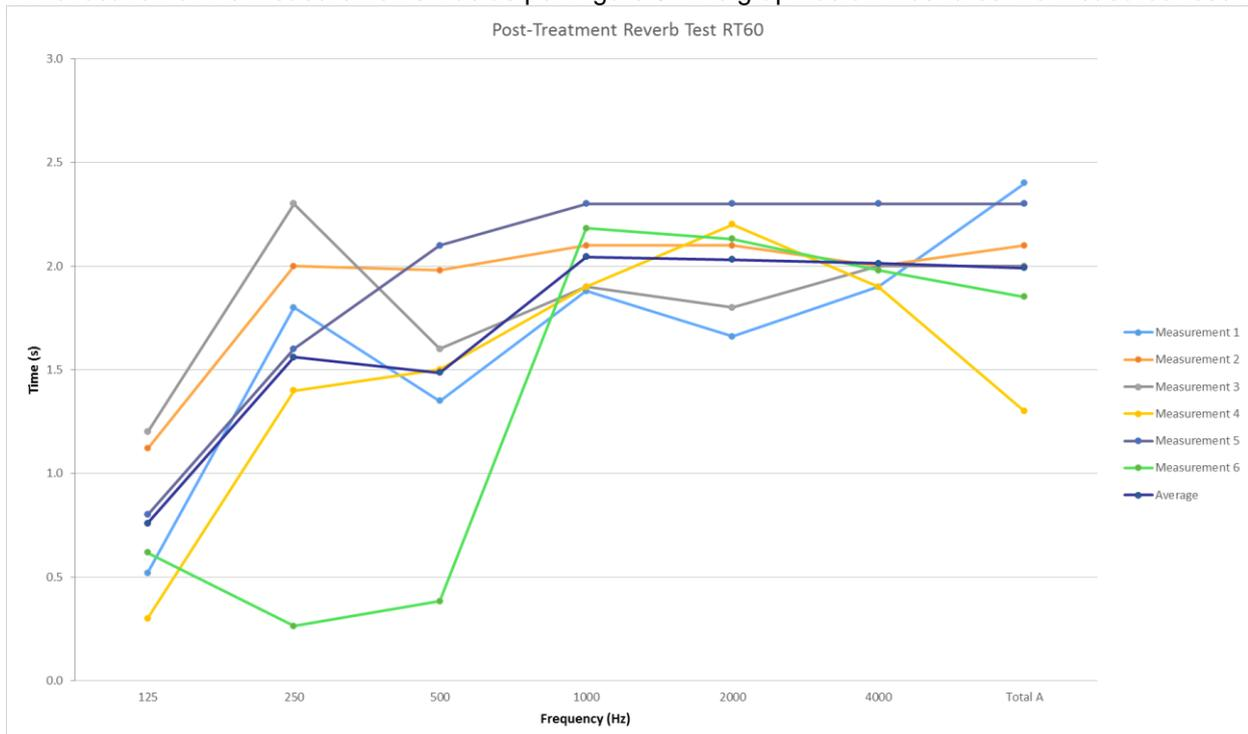
Post treatment reverb measurements have an average result of 2.0s as an overall reverb time. This exceeds the criteria of 1.44s, however, the hanging baffles have eliminated any standing waves and flutter echoes in the large corners of the building. This is a significant decrease in RT from 3.1s to 2.0s.
