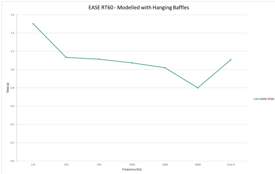
The graph above illustrates the RT results after modelling in EASE. This assumes 45 hanging baffles hanging 4.5m above the ground, humidity 60%, internal ambient temperature of 20Deg Celsius and 1013 hPa. The results show exceptional performance of the hanging baffles. This is in line with the 1.44s reverb time criteria. However Pre-Test measurements and the empty swimming pool showed vast difference in the modelling and testing data.
