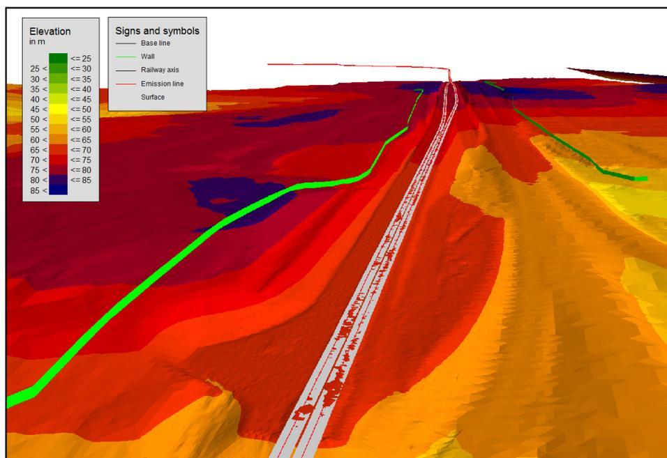
Figure 3: Terrain model snapshot with noise barriers
