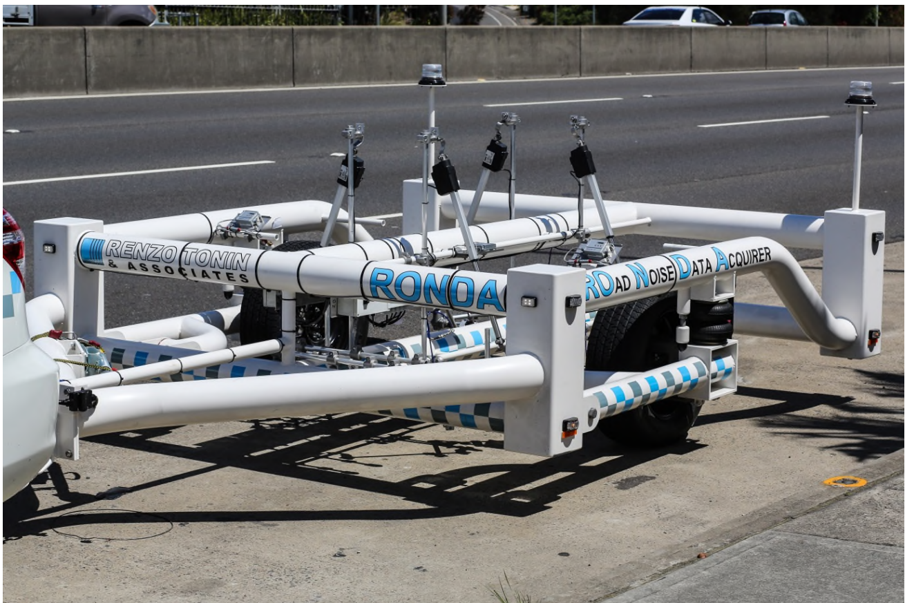
Figure 1: CPX Trailer RONDA Open Frame Design
