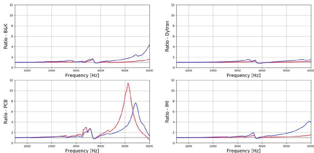
Figure 6: Dynamic Mass Shaker Results: Flat Magnet (blue) and Dual Rail Magnet (red) relative to Stud Mount, 500 Hz to 6000 Hz
