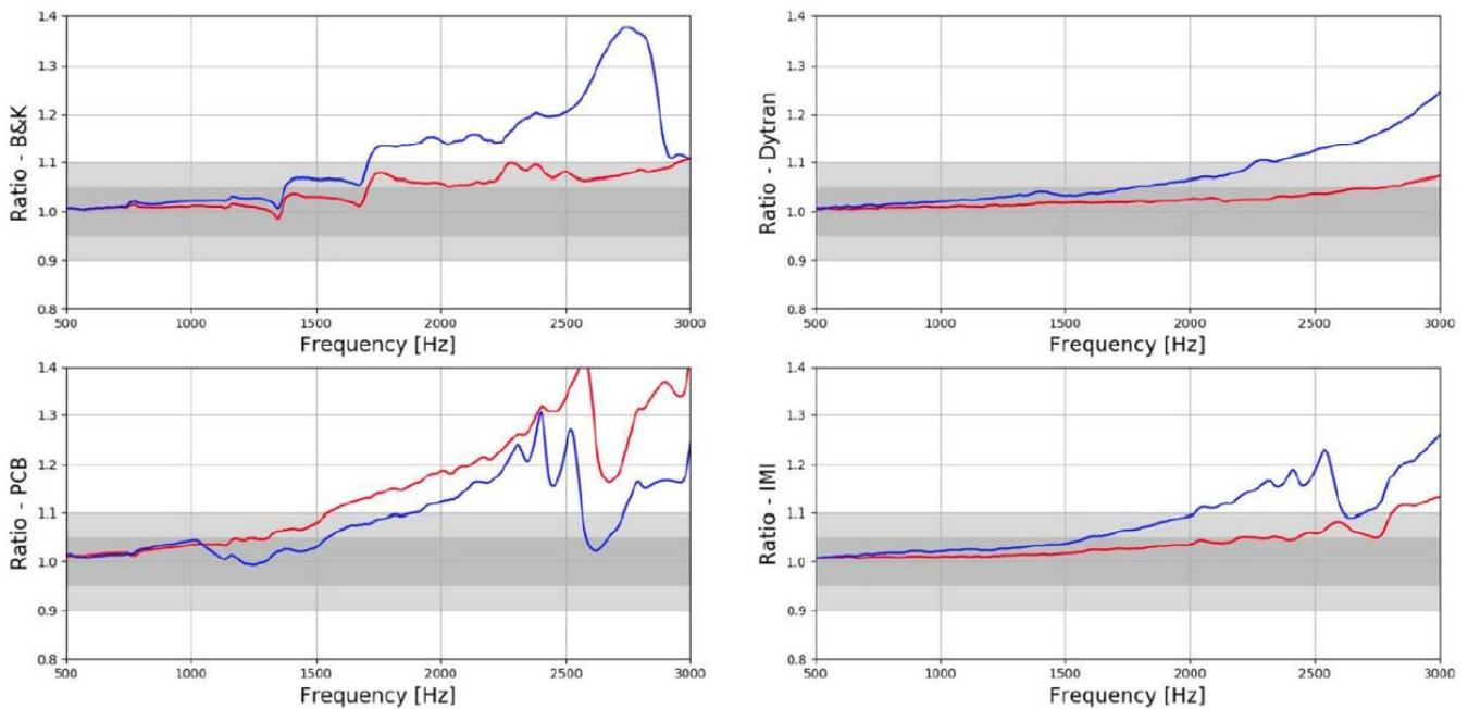
Figure 5: Dynamic Mass Shaker Results: Flat Magnet (blue) and Dual Rail Magnet (red) relative to Stud Mount, 500 Hz to 3000 Hz
