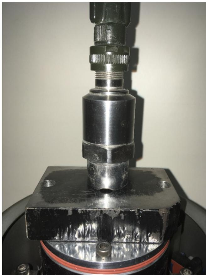
Figure 4: Test Configuration – PCB 393A03 Accelerometer on Dual Rail Magnet (strain relief not shown)
