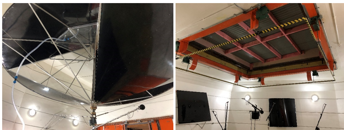
Photograph 5 (left): The rainfall system mounted above the frame within a diffuser Photograph 6 (right): The lower receiving chamber, displaying the underside of a system and the frame
