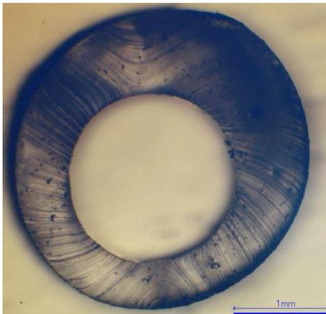
Figure 1: A cross sectional view of the PDMS microfluidic channel.
