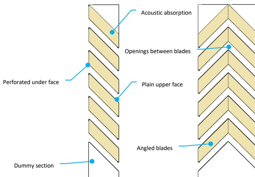
Figure 2: Design features of a typical acoustic louvre for a single stage (left) and two-stage (right) louvre
