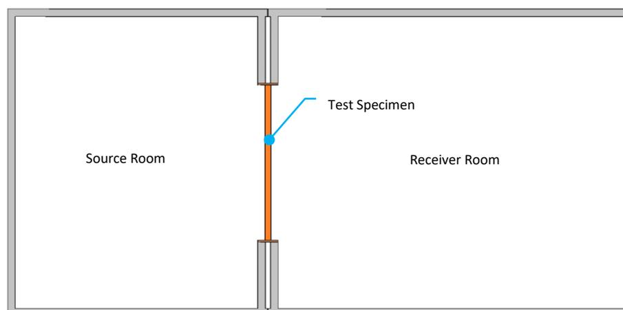
Figure 4: Transmission loss suite for reverberant to reverberant testing
