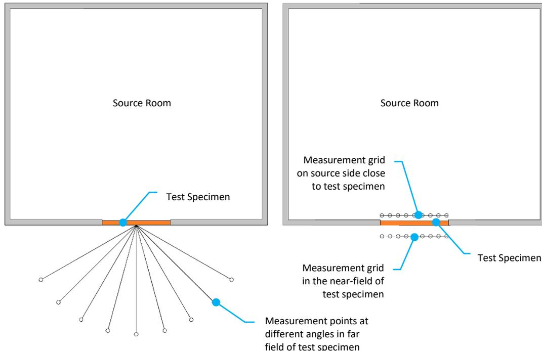
Figure 5: Test configurations for reverberant to free-field testing. The left side shows insertion loss test arrangement while the right side shows noise reduction test arrangement
