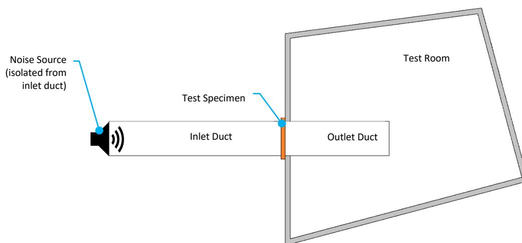
Figure 6: Schematic of the in-duct test configuration. The test room can be either a reverberation chamber for the diffuse field method or free-field (anechoic room or external to building).
