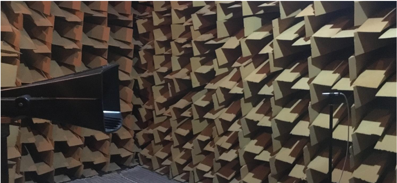
Figure 6: Loudspeaker testing in the anechoic chamber at The University of Auckland
