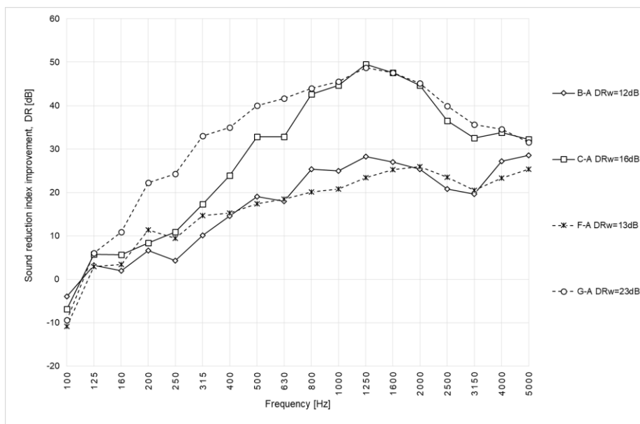
Figure 5: One side or two side linings comparison
