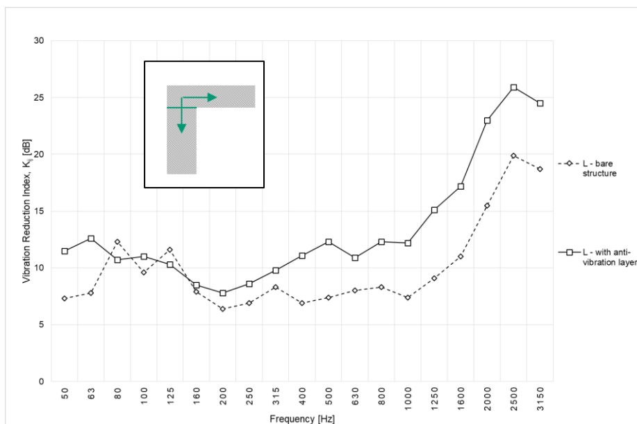
Figure 7: Vibration reduction index K_{ij} - L Junction
