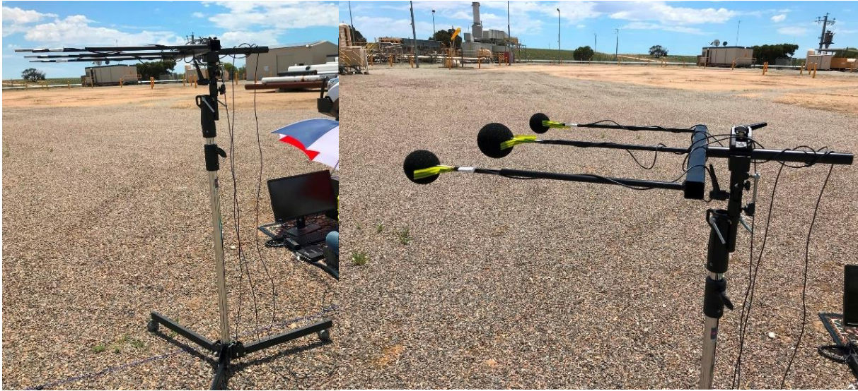
Figure 3: Microphone apparatus arrangement. Left: without wind socks. Right: with wind socks.
