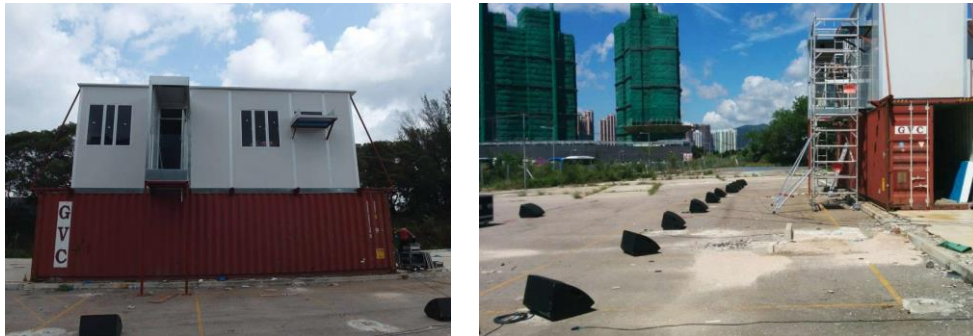
Figure 4: Offsite mock-up room and the line of loudspeakers (case 2)
