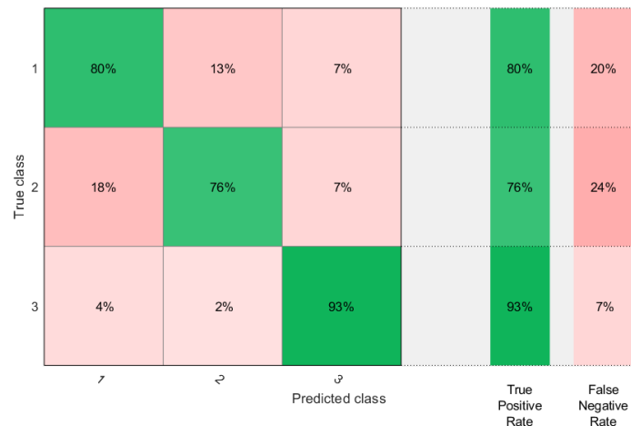
Figure 15: Cubic SVM Model Accuracy for Variable RPM
