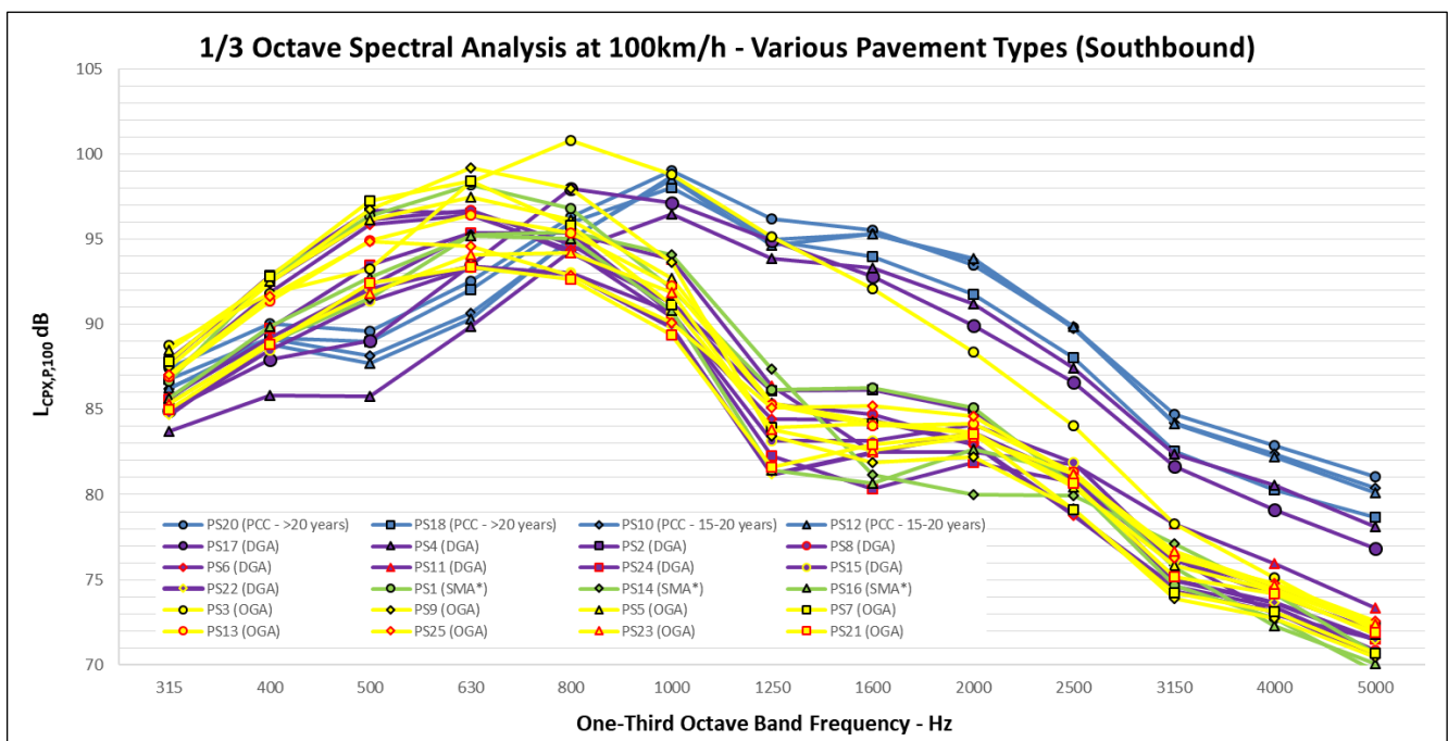
Figure 6: One-Third Spectral Analysis at 100km/h Reference Speed for Various Pavement Types (Southbound)
