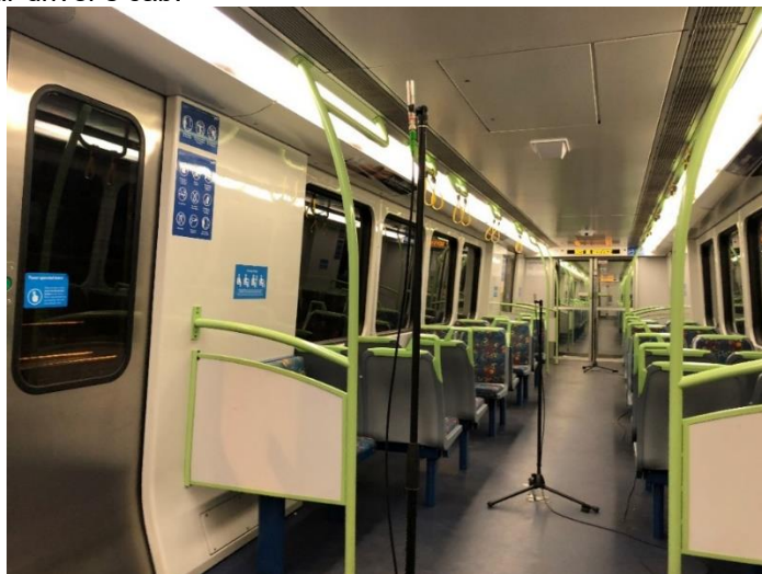
Figure 8: In carriage noise level measurement locations within X'Trapolis rolling stock.
