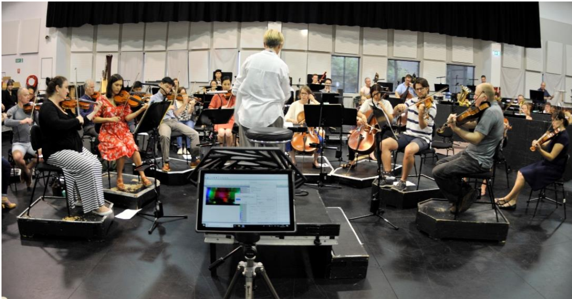
Figure 1: Hand held acoustic camera mounted to tripod during a rehearsal
