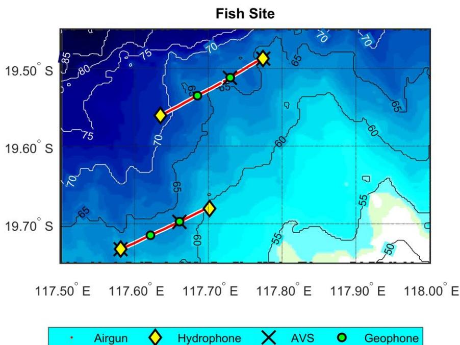
Figure 3: Bathymetry (in metres), sensor deployment and airgun shot locations for the Fish-1 (upper trace) and Fish-2 (lower trace) data sets
