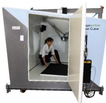
Figure 2 – Alpha Cabin: a compact reverberation room for sound absorption measurement
