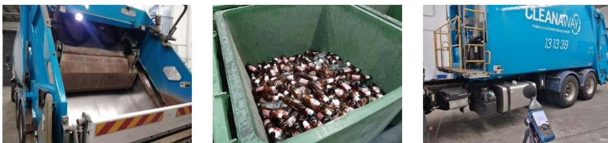
Figure 2 – The Rear Loader rubbish truck, the bin with 750 glass bottles and the microphone set-up
