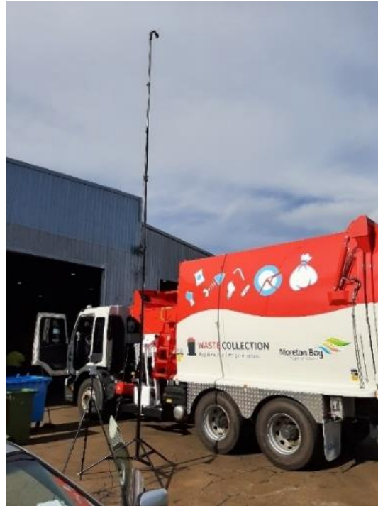
Figure 9 – Side Loader rubbish truck and the noise measurement set-up
