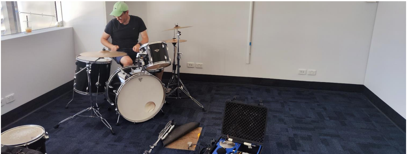
Figure 4 – Carpet in the source room at the 450 mm position with full drum kit and mounted vibration monitor on concrete.
