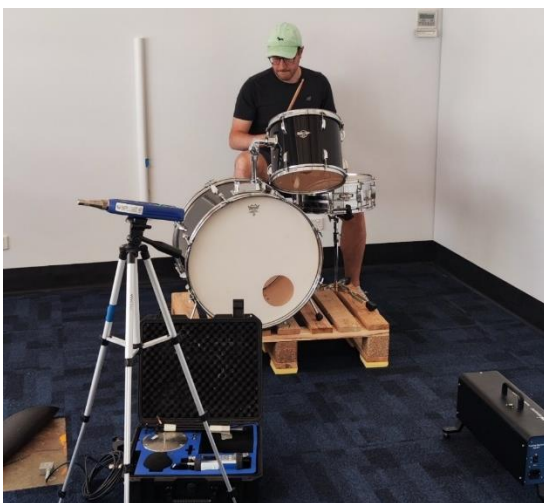
Figure 5 – Position on 180 mm of concrete with platform.
