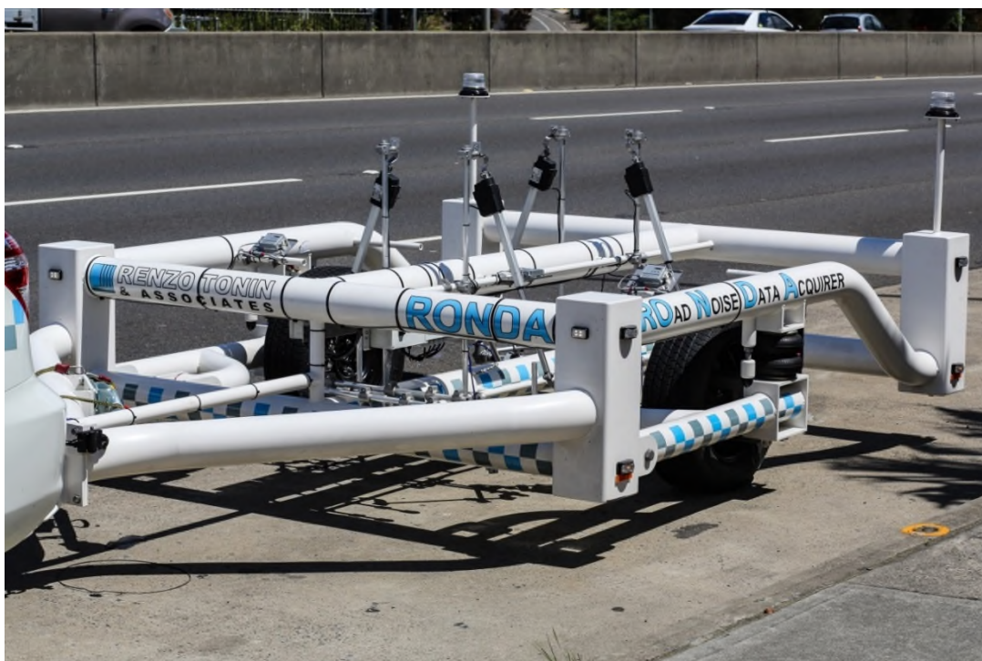
Figure 1: CPX Trailer RONDA Open Frame Design
