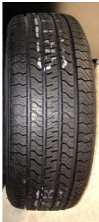
Figure 2: 16" SRTT Tyre and Tread Pattern
