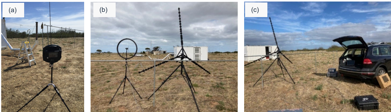
Figure 13 – Acoustic cameras (a) SoundCam (Resonate), (b) gfaitech ring array and star array, (c) gfaitech star array (HW Technologies).
