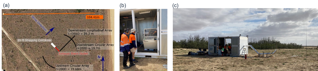
Figure 11 – (a) Geometry of the test site, showing shipping container, exhaust duct, linear and circular microphone arrays, (b) SR-30 turbojet engine on startup, (c) genset shipping container, and exhaust.
