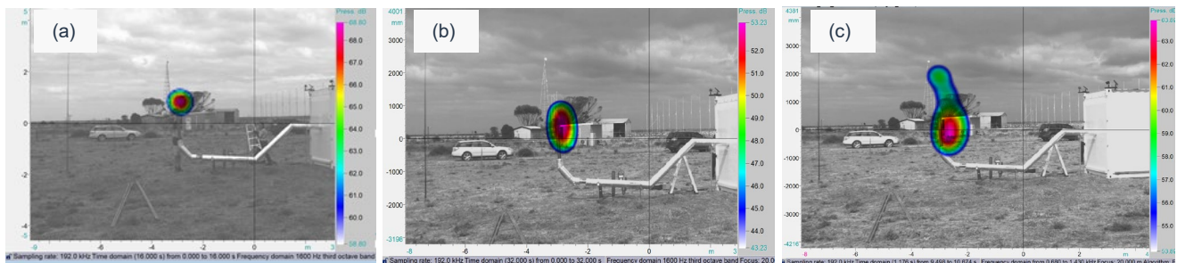
Figure 14 – Acoustic field observed by the 48 microphone gfaitech ring array. (a) 50mm compression driver: SPL 1.6 kHz one-third octave band, (b) hot exhaust stack with the turbine operating at 43,800 RPM: SPL 1.6 kHz one-third octave; and (c) “bubbles” of sound observed from turbine exhaust when wind gusts are present: SPL 1 kHz octave band.
