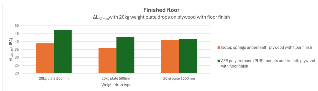
Figure 5 – The delta L_{AFmax} comparison of springs and PUR mounts underneath the platform with a floor finishes
