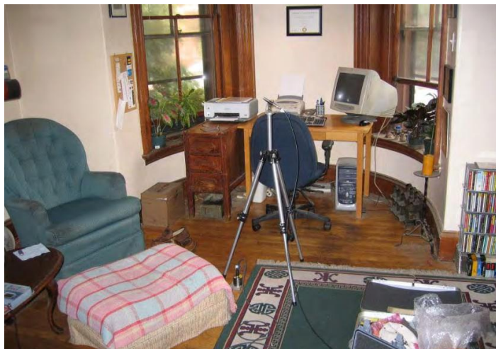
Figure 1: Typical direct ground-borne noise monitoring setup (Zapfe TCRP D-12 , 2005)
