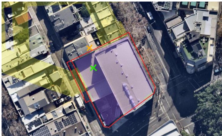
Figure 6: Aerial view of attended noise measurement. Green 'x' indicates location of construction activities (30m underground), orange 'x' monitoring location at sensitive receiver
