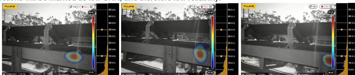
Figure 9: series of Acoustic images showing Motion of reflection relative to conveyor
