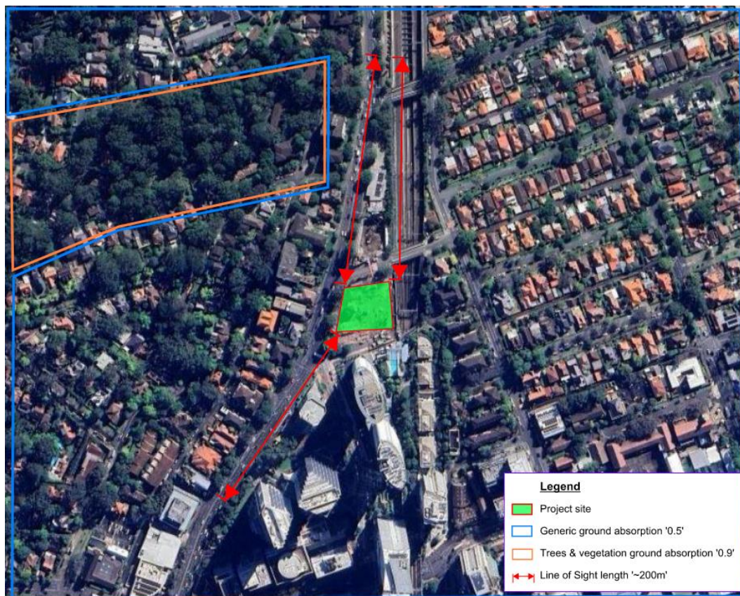
Figure 1: Markup for ground absorption and LoS criteria
