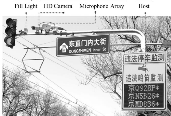
Figure 3 – Example of the Motor Vehicle Horn Detection and Capture System in Beijing, China [“Figure 1: Composition of the Horn-Capturing System for Motor Vehicles” in (Niu et al., 2020)]
