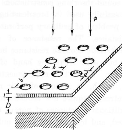
Figure 1: Micro-perforated panel absorber (MPA) according to (Maa, 1975) where  $d$  is the orifice diameter,  $b$ , the distance between orifices,  $t$ , panel thickness and  $D$  air cavity depth, between panel and backing wall.
