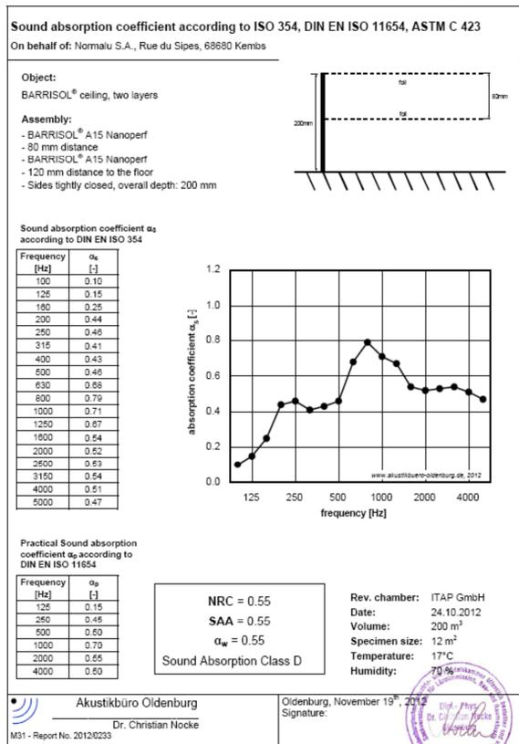
Figure 10: Results from laboratory tests for different set-ups.
