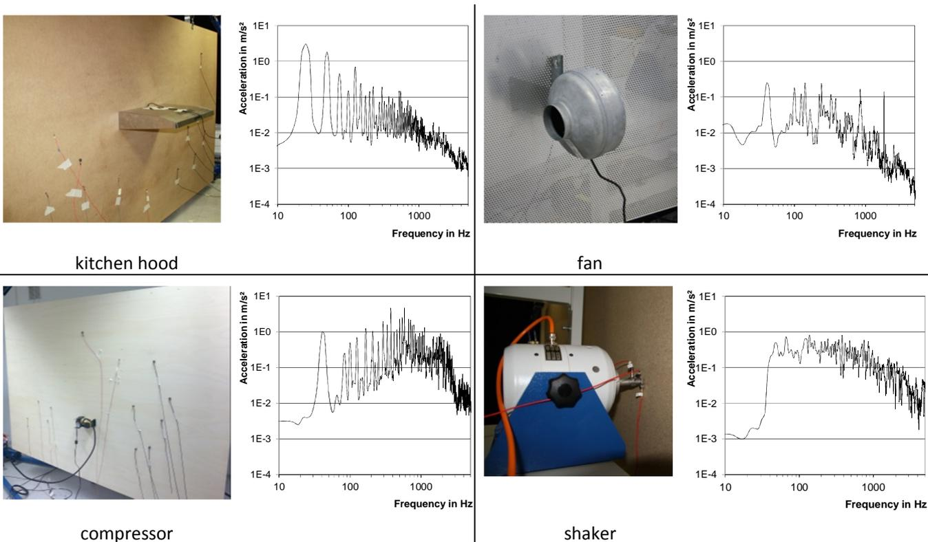
Figure 2: Used structure-borne sound sources and acceleration spectra – 8 mm MDF
