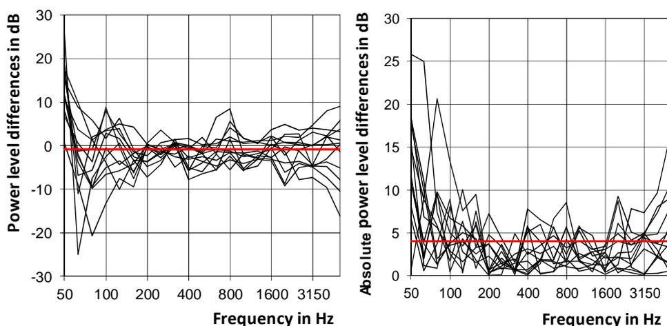
Figure 3: Differences between measured and predicted power – red line represents the mean (Vogel, 2015)
