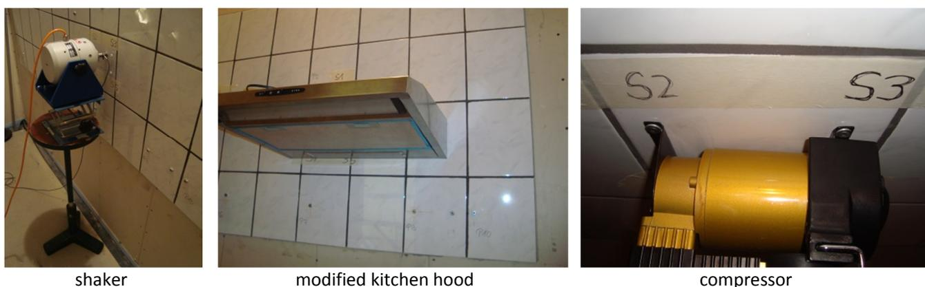
Figure 4: Structure-borne sound sources in the source room ( $V = 35 \text{ m}^3$ ) (Vogel, 2016)
