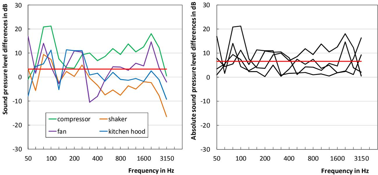
Figure 5: Difference of the normalised sound pressure level – calculated minus measured values, red line represents the mean (Vogel, 2016)
