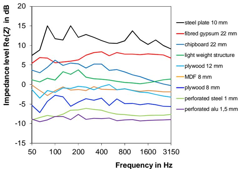
Figure 1: Measured point impedance of the reception plates used
