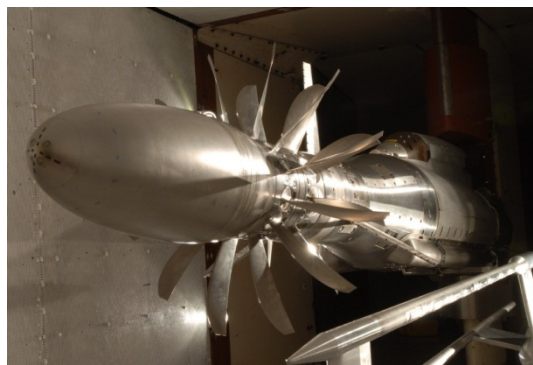
Figure 5: Rolls-Royce's 1/6th scale open rotor rig installed in the ARA wind tunnel in Bedford, UK. Picture courtesy of Rolls-Royce plc.
