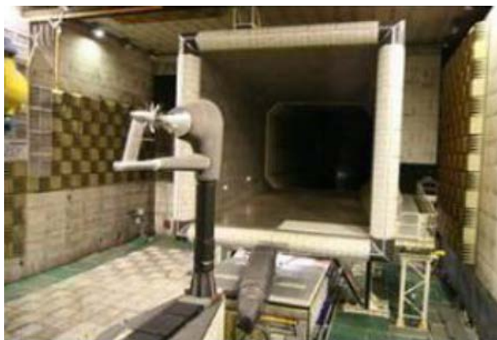
Figure 2: Testing of a 1/6 th scale open rotor rig in the DNW wind tunnel with pylon installed upstream. Picture taken from Parry et al. (2011)
